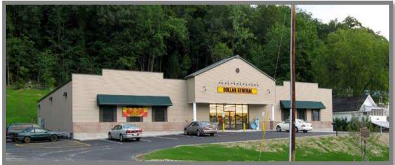
Figure 1: Use of Fenestration to break up a long expanse of blank wall.
